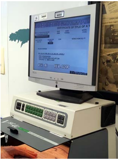
The document examination device magnifies and illuminates the questionable title for an in depth examination
